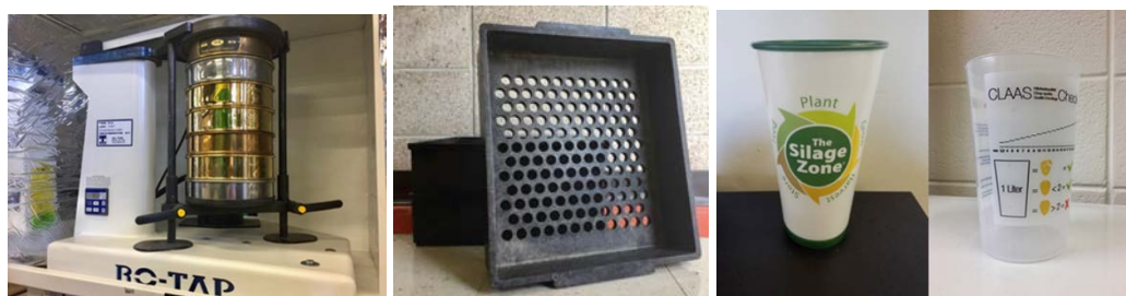
Figure 1. Typical methods of assessing corn kernel particle size in chopped and processed corn silage. From left to right: 1) Ro-Tap™ Sieving, 2) Penn State Particle Separator, 3) One liter cups.
